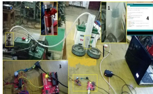
Fig 2 Fuel premixing system Fuel pump and fuel tank [1], Fuel injector [2], Injector control circuit [3], Program for electronic circuit [4]
